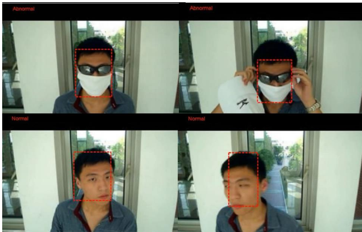
Figure 2.9 Examples of face occlusion detection results [13]
