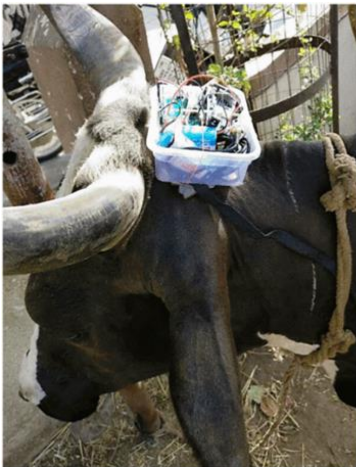
Figure 2.6.2.2 Hardware module attached to the animal [20].
