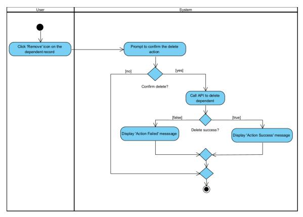
Figure 3.10 Activity diagram for delete dependent
