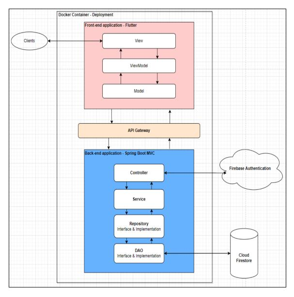
Figure 3.1 Architecture diagram of the system
