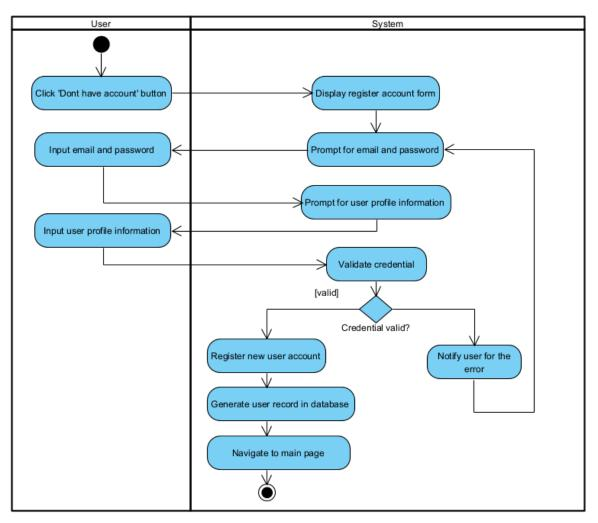
Figure 3.4 Activity diagram for register account
