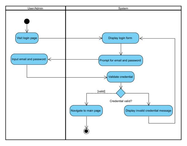
Figure 3.3 Activity diagram for login to system
