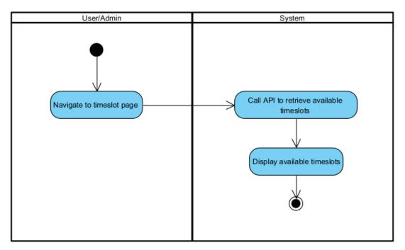
Figure 3.15 Activity diagram for view available timeslot
