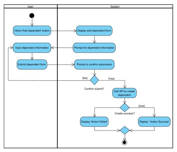
Figure 3.7 Activity diagram for create dependent
