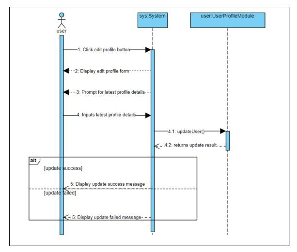
Figure 4.11 Component interaction diagram of update profile
