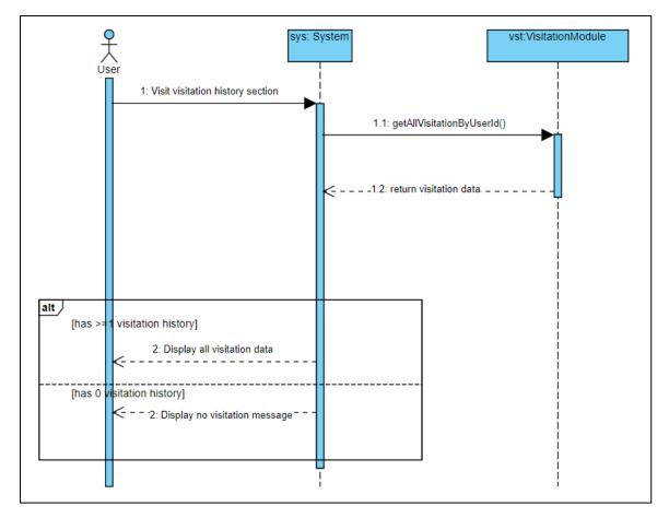
Figure 4.23 Component interaction diagram of view visitation record
