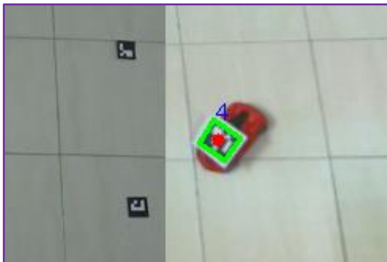
Figure 3.2.3.3 Marker detected and bounded (*the other two markers are from a different class and so is discarded)
