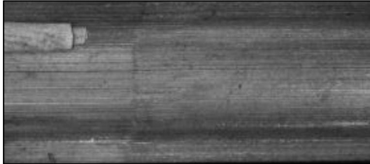
Figure 3.1 Defective magnetic tile with a cluttered surface.
