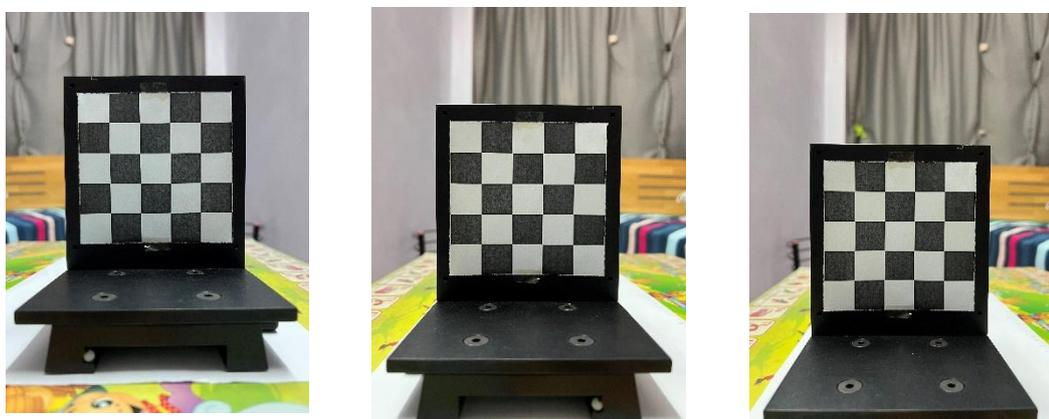
**Figure 4.1: Checkerboard Images with 60cm, 70cm, 80cm Camera's Height (Left to Right)**
