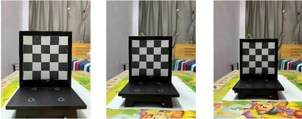
**Figure 4.2: Checkerboard Images with 20cm, 25cm, 30cm Camera's Distance (Left to Right)**
