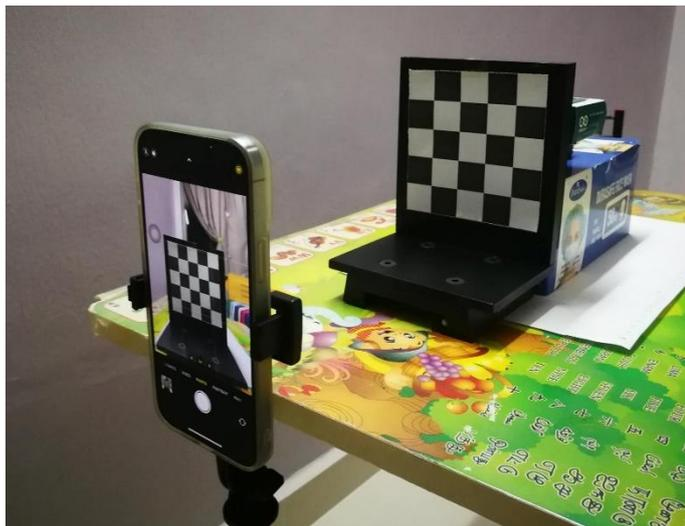
**Figure 3.5: Hardware Configuration for Camera Calibration System.**
