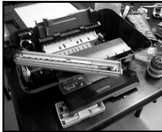
Figure 2.7: Disassembled slider from HP inkjet printer (Kang, 2016)
