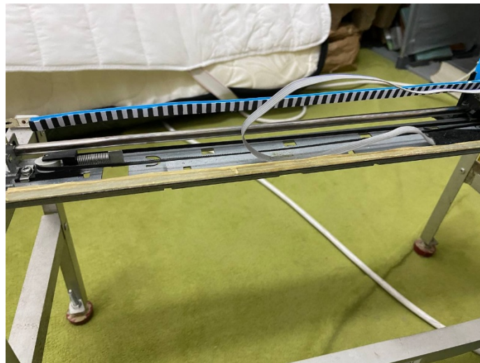
Figure 4.3: Replace a new encoder strip
