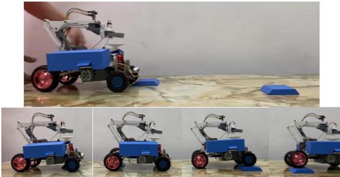
Figure 4.18: The prototype passes two barriers on the left and right sides (side view)
