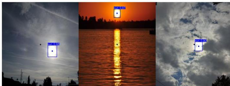
Figure 4.10: Detection of the Sun at different situations. From left to right: (Left) Detection of Sun during sunny day, (Middle) Detection of Sun during sunset, (Right) Detection of Sun when partially blocked. The value beside the class ‘Sun’ is the confidence level of the detection algorithm, which is over 90% for each case.
