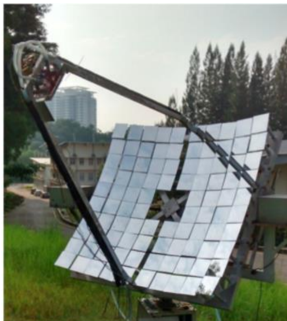
Figure 2.1: The previously constructed prototype of dense array concentrator photovoltaic (DACPV) at TARUC, Setapak (Chong et al. , 2017). The DACPV prototype consisted of a non-imaging dish concentrator (NIDC) and a DACPV receiver.
