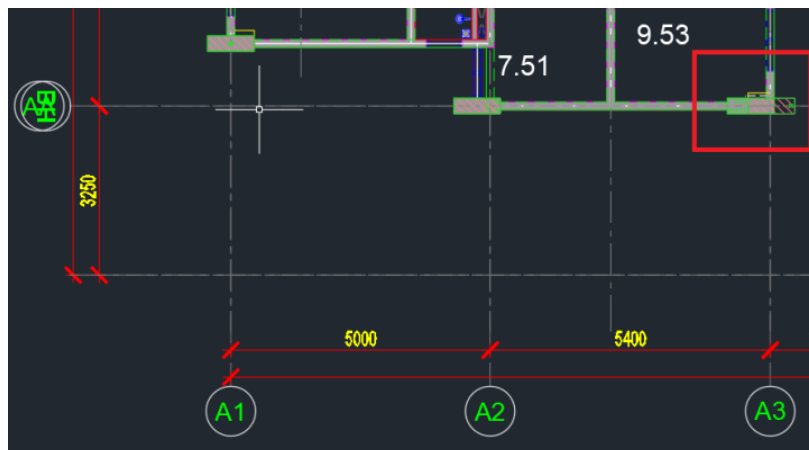
Figure 3.14: Issue of placing the structural column.
