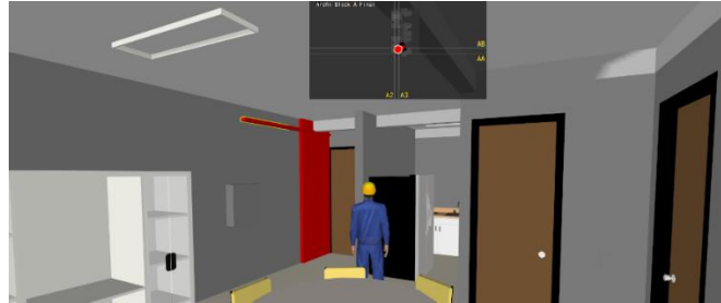
Figure 3.33: Clash detected between electrical wire and structural column.
