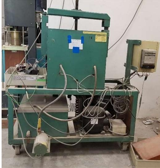
Figure 3.22: Set-up of thermal conductivity testing equipment.
