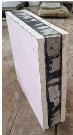
Figure 3.15: Sized-down wall panel utilizing gypsum board as skin layer.
