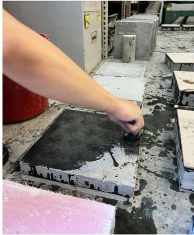
Figure 3.14: Epoxy resin is being applied to the surface of the concrete core.
