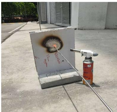
Figure 3.18: Commencement of flame exposure test on a wall panel specimen.
