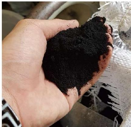
Figure 3.6: Powdered crumb rubber.
