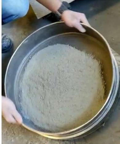
Figure 3.9: Sieving of ‘Orang Kuat’ branded OPC with 600  $\mu\text{m}$  screen.
