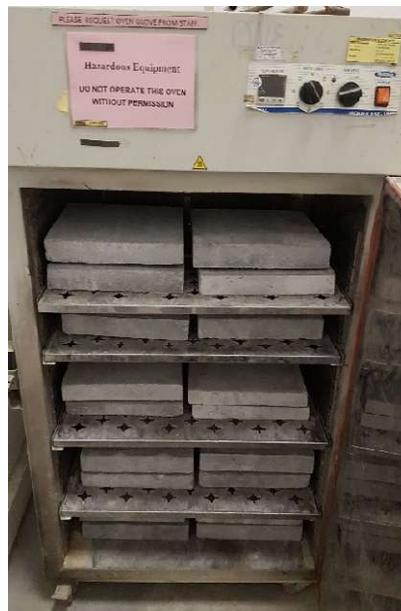
Figure 3.12: Oven-dried concrete cores in a furnace.
