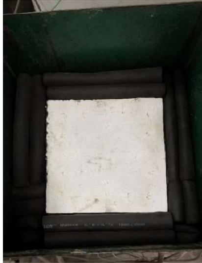
Figure 3.20: The specimen is covered with wools before the test.
