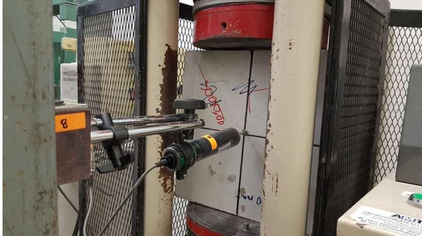
Figure 3.16: Set-up of the load-bearing capacity test on vertically positioned sandwiched wall panel.
