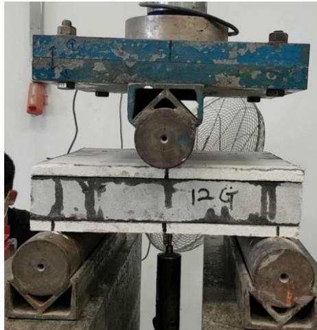
Figure 3.17: Set-up of the flexural strength test on a sandwiched wall panel.
