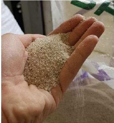
Figure 3.5: Oven-dried fine aggregate.
