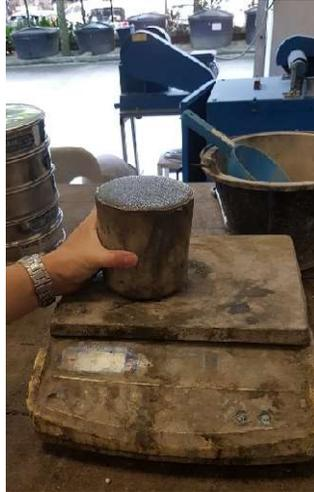
Figure 3.11: Density test of fresh concrete.
