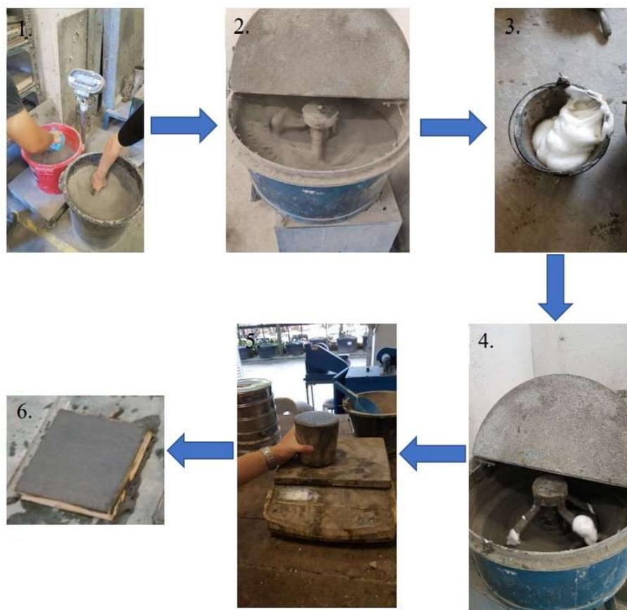
Figure 3.10: Mixing procedure of rubberized lightweight foamed concrete.
