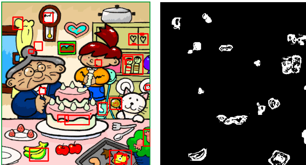
Figure 4.9: Bounding Boxes on Differences on Modified Image (Left) and Thresholding to Accentuate Modified Parts (Right).
