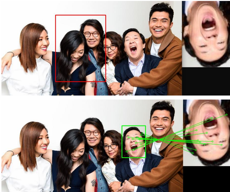
Figure 2.6: Results for Template-based Approach (Top) and Feature-based Approach (Bottom) for Rotated Template Image (Luces, 2019).
