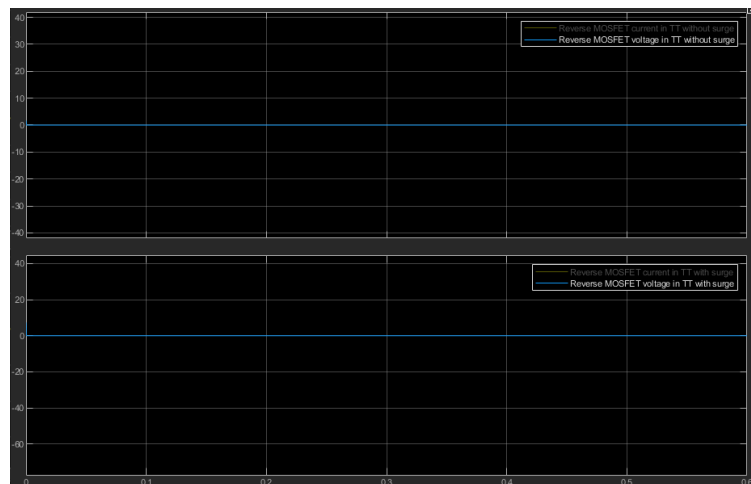
Figure 4.26: Voltage of reverse MOSFET with and without surge
