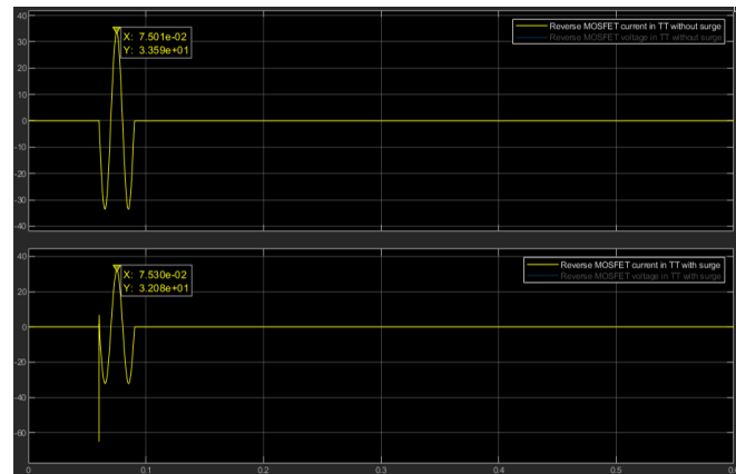
Figure 4.27: Operating current waveform of reverse MOSFET with and without surge
