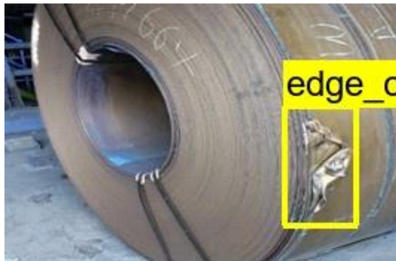
Figure 4.5 : Example of an output image with edge crack defect
