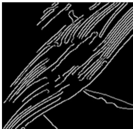
Figure 3.14 : Output of Canny Edge Detection for Edge Defect
