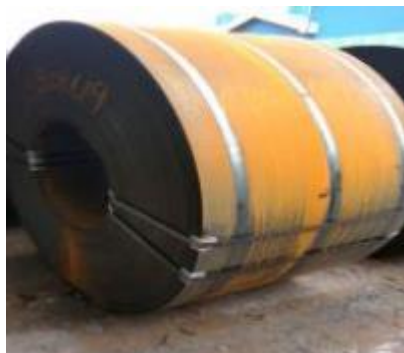
Figure 3.8 : Sample Input Image of Rusty Hot Rolled Steel
