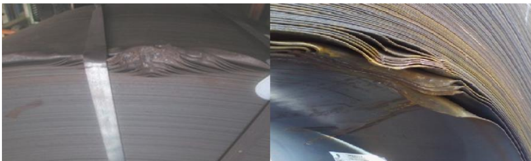
Figure 4.6 : Images of edge folded defects taken from different distances
