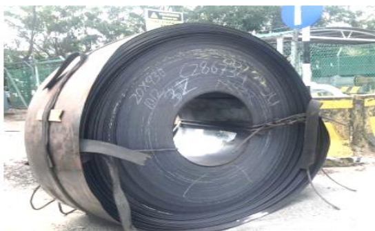
Figure 3.15 : Hot rolled steel with Loose Wrap issue
