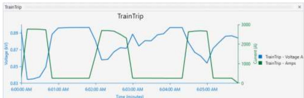
Figure 4. 8 Non-regenerative train voltage vs current
