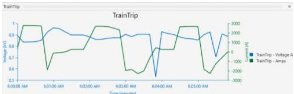
Figure 4.20 Regenerative train voltage vs current
