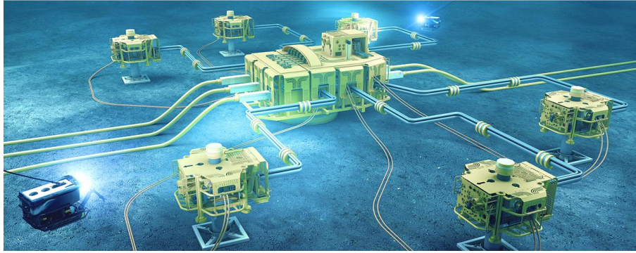
Figure 2.9: Subsea Production Systems (AkerSolutions, n.d.)
