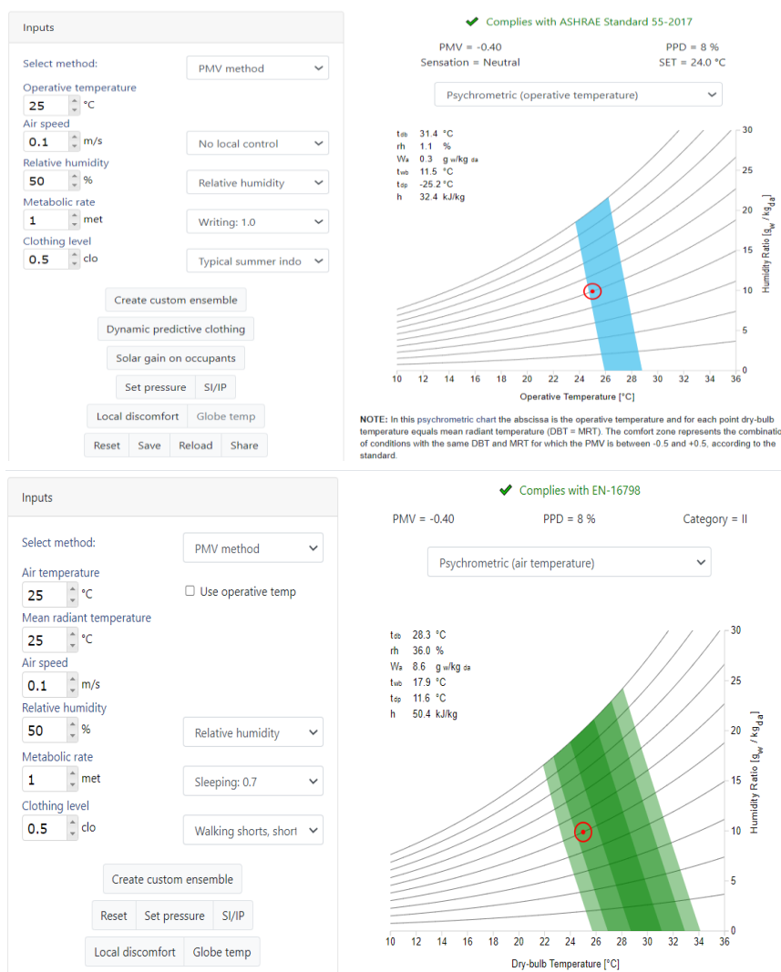
Figure 3.53: Thermal Comfort Tool following ASHRAE-55 (A) And EN-16798(B) at the same weather conditions
