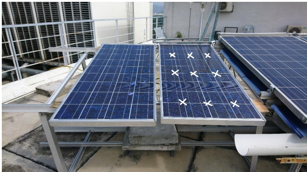
Figure 11: The two panels being used, left: reference panel, right: panel with cooling (the 9 crosses represent the temperature collection points)
