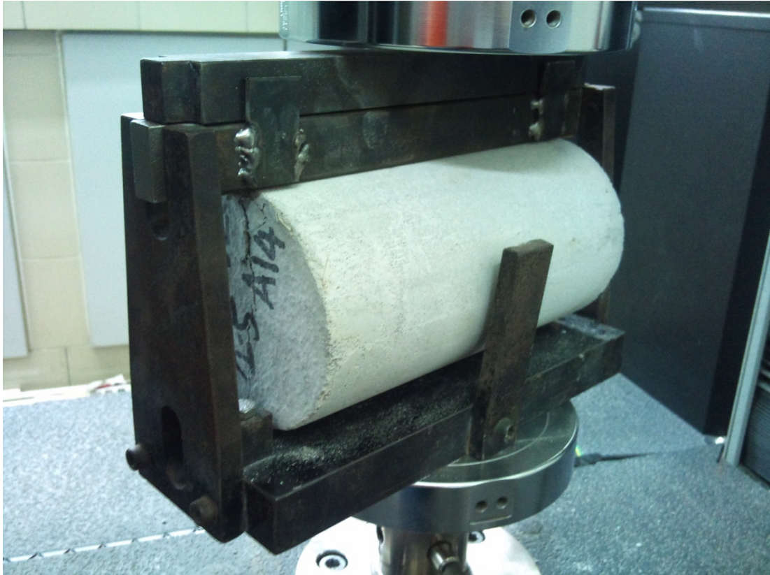
Figure 3.8: Splitting Tensile Strength Test of Lightweight Foamed Concrete
