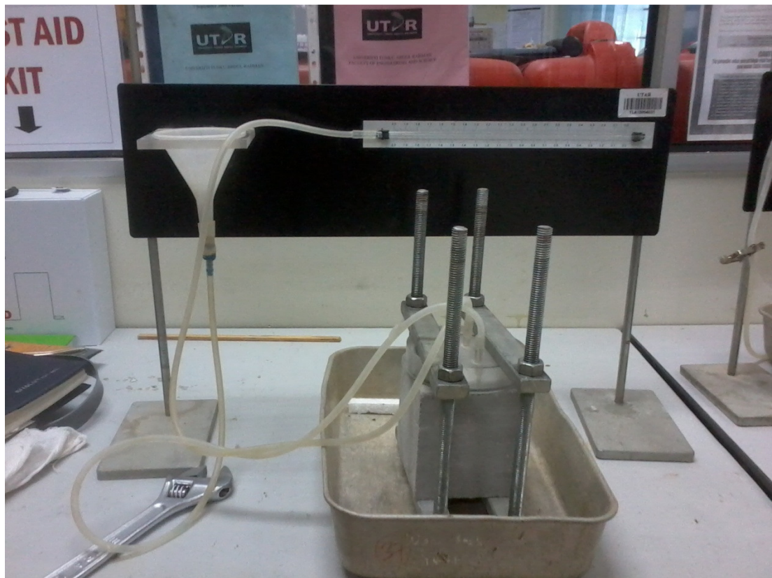
Figure 3.12: ISAT of Lightweight Foamed Concrete
