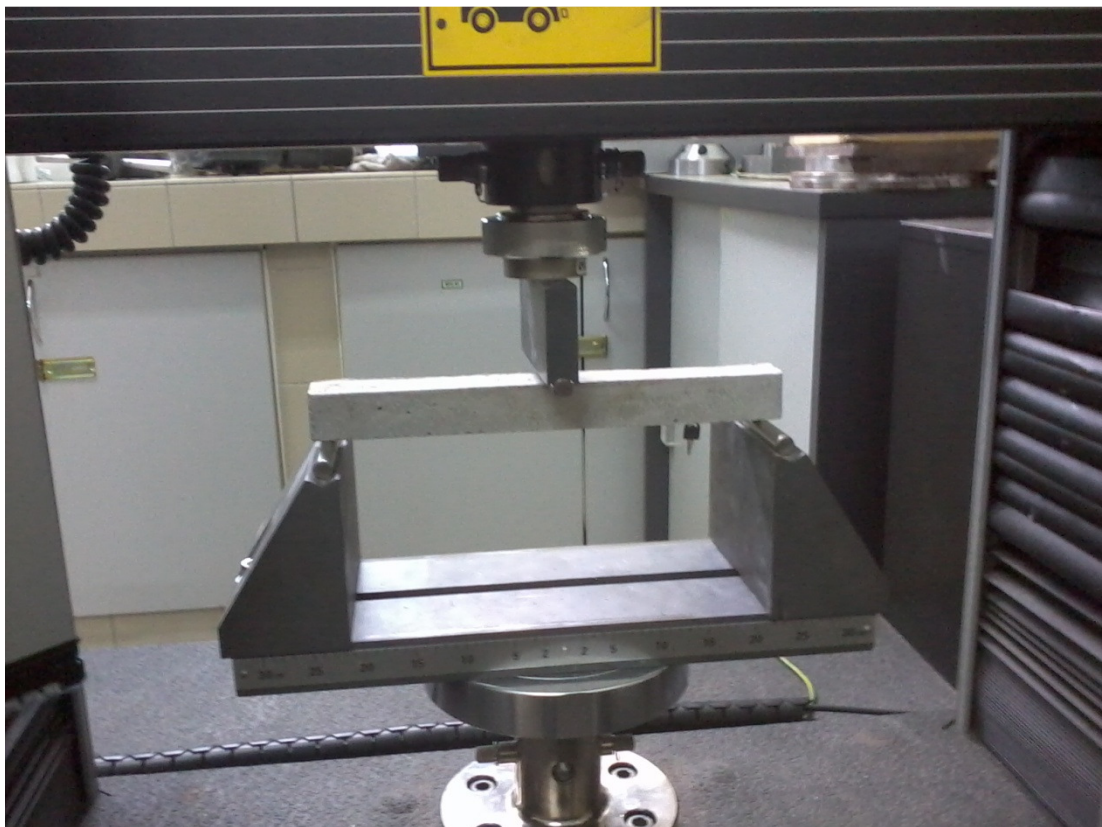
Figure 3.9: Flexural Strength Test of Lightweight Foamed Concrete
