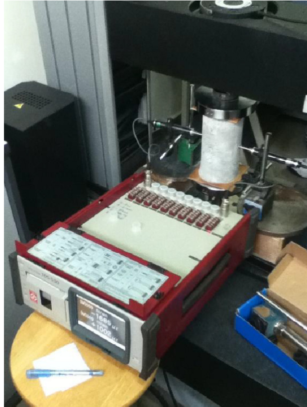
Figure 3.10: Poisson's Ratio Test of Lightweight Foamed Concrete
