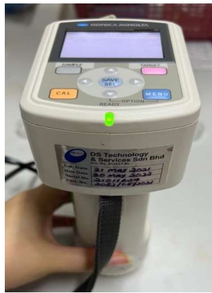
Figure 3.6: The colorimeter was used to measure the egg yolk colour index.
