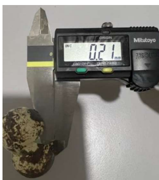
Figure 3.5: The digital calliper was used to measure the eggshell thickness.
