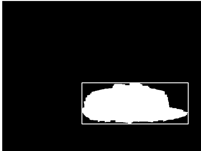
Figure 4. 8: Contour detected by OpenCV findContours function
