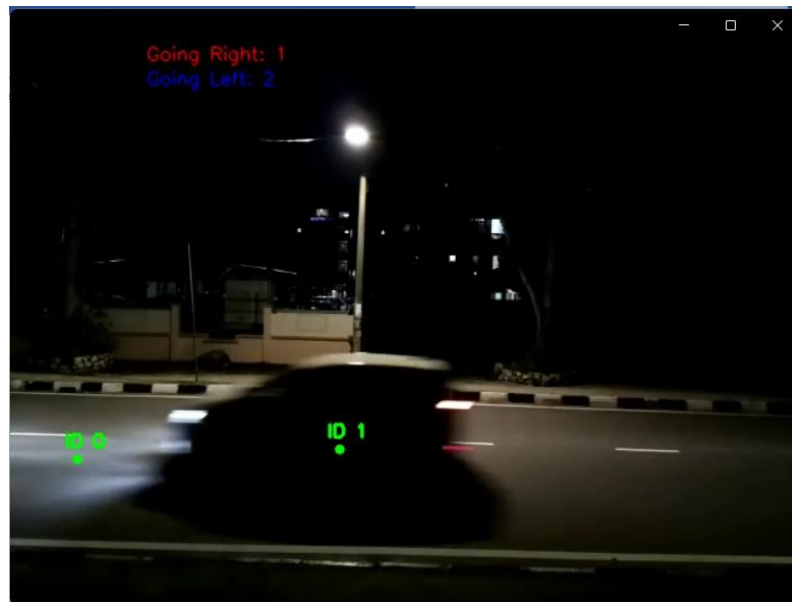
Figure 4. 35: Detection error when scene is dark
