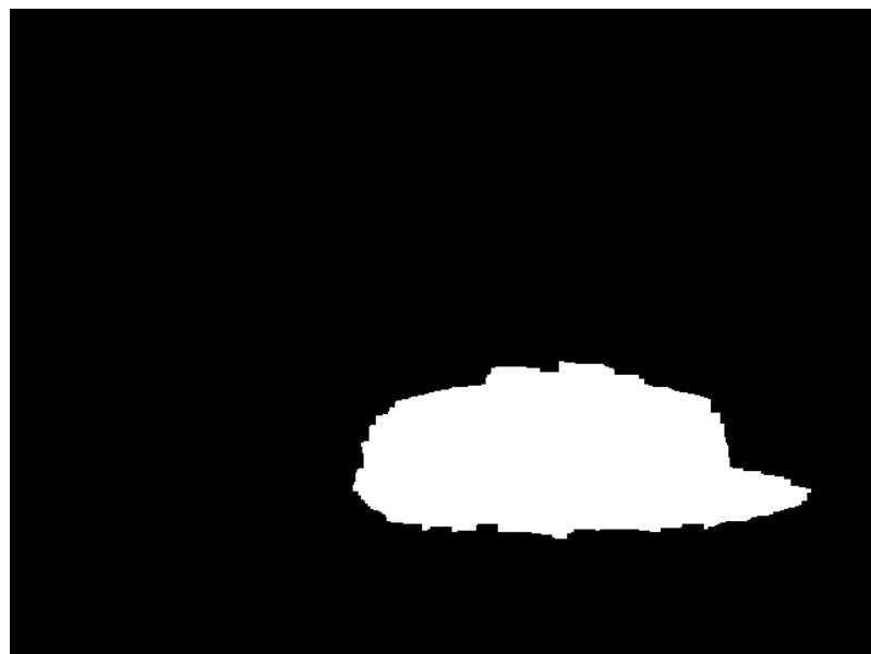
Figure 4. 6: Frame after applying Morphology Opening
