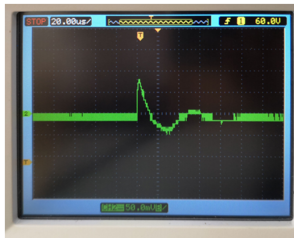
Figure 94: Response time of MOSFET
