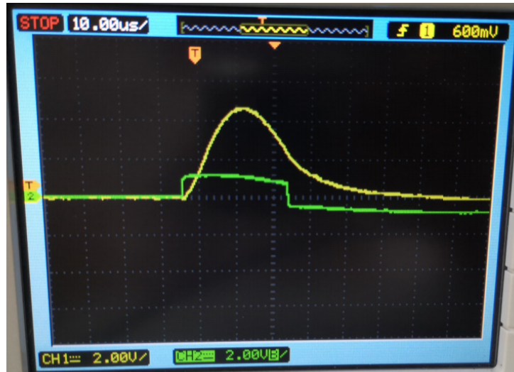
Figure 85: Clamping waveforms of MOV
