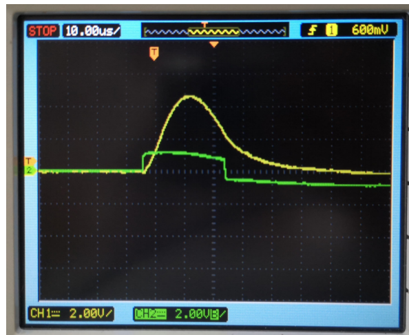
Figure 93: Response time of MOV
