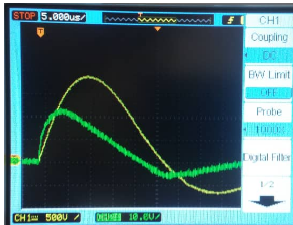
Figure 88: Clamping waveform of MOSFET
