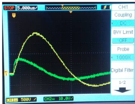
Figure 89: Clamping waveform of IGBT
