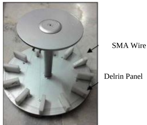
Figure 2.2: Stewart Platform with Shape Memory Alloy [7]
