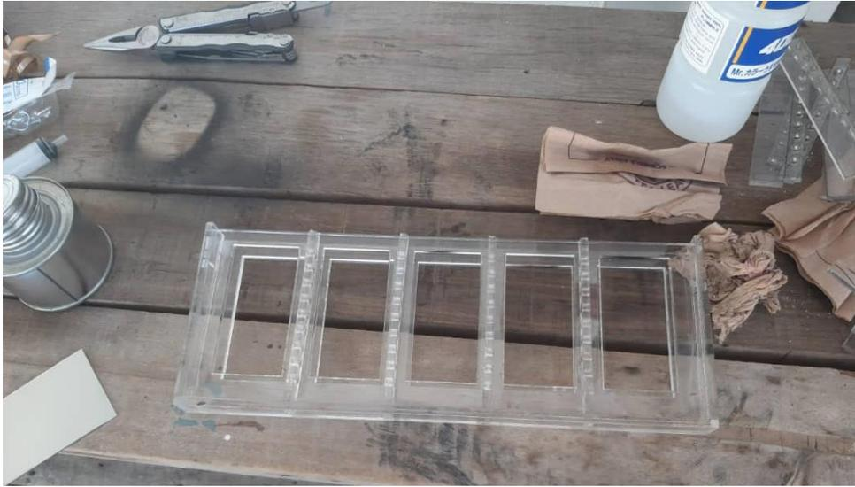
Figure 4-5 join fusion of acrylate sheet by using chloroform
