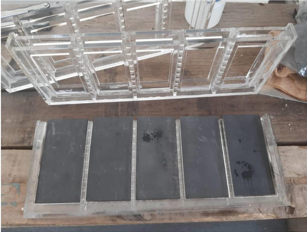
Figure 4-6 try fit of machined graphite sheet into fused acrylic housing
