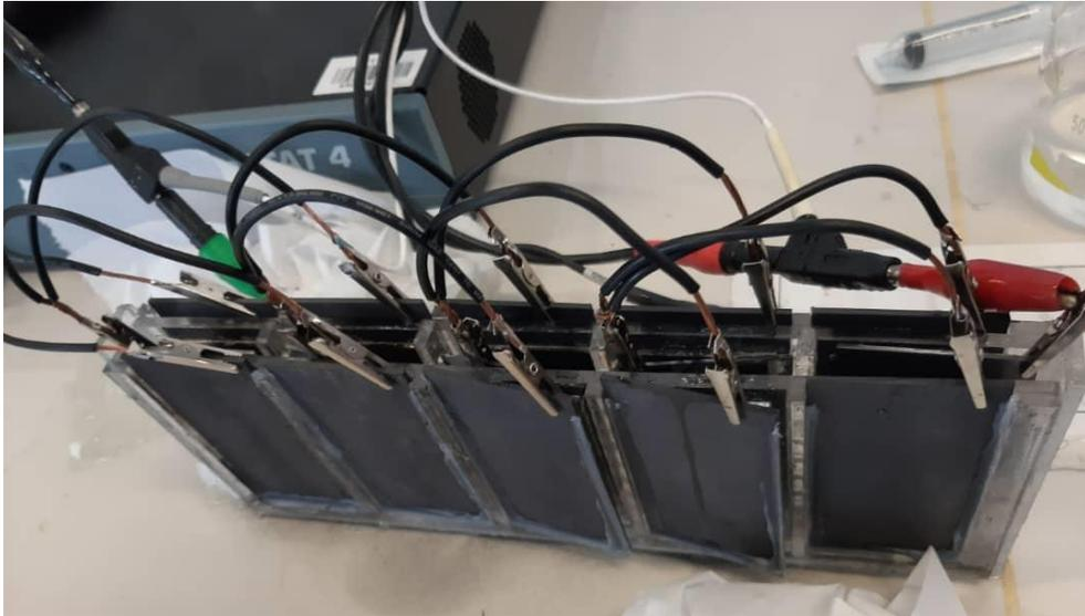
Figure 4-14 sealant fail during test
