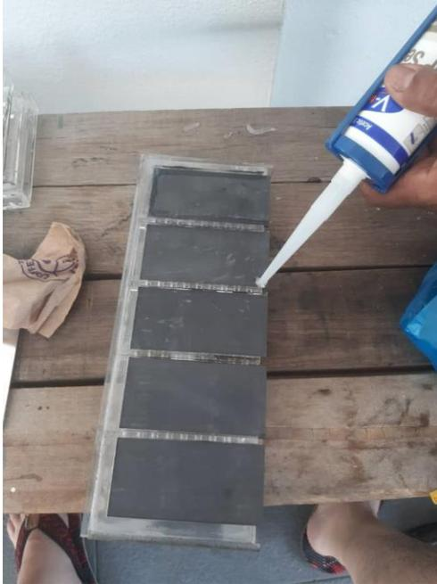
Figure 4-7 application of silicone sealant to hold graphite sheet in place
