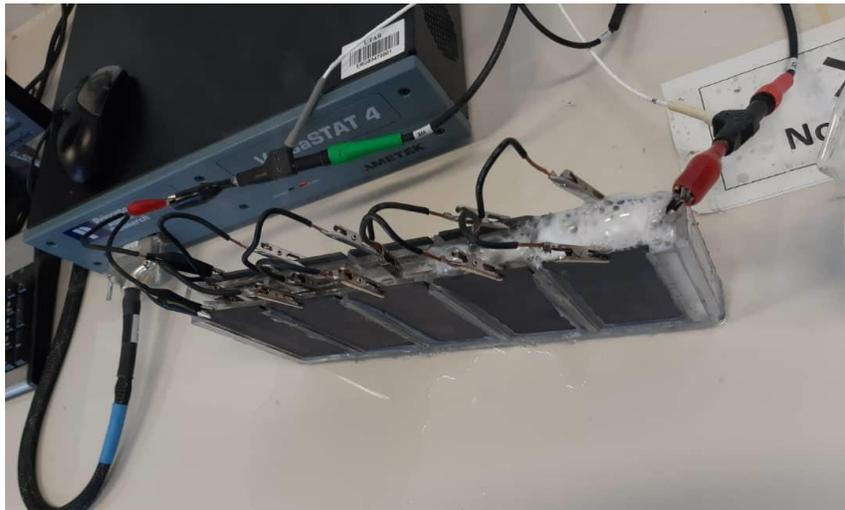
Figure 4-13 after load the cell with electrolyte connected the cell with VersaSTAT 4 Potentiostat Galvanostat, bubble form during the test, may cause by formation of hydrogen gas or boiling of electrolyte or both.
