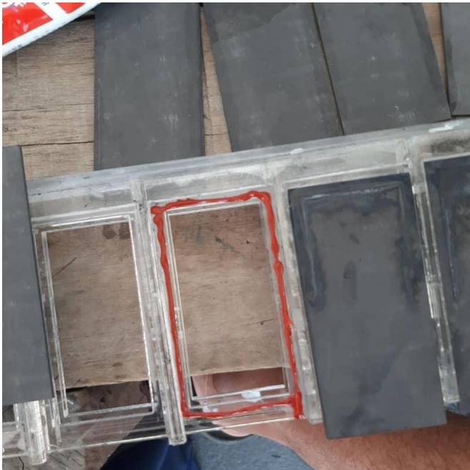
Figure 4-16 application of gasket
