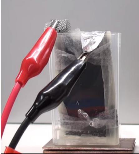
Figure 3-3 simple design of a single cell
