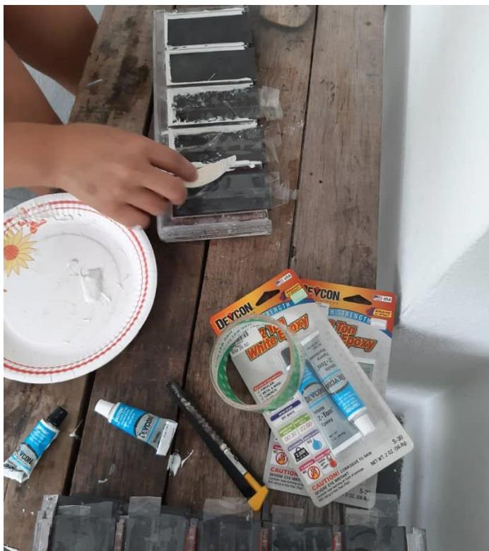
Figure 4-17 application of epoxy sealant on the graphite with gasket beneath.
