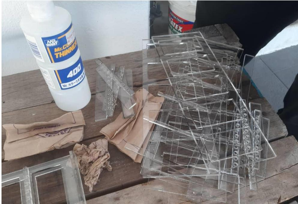
Figure 4-4 cleaning and surface preparation before joining of the acrylate sheet
