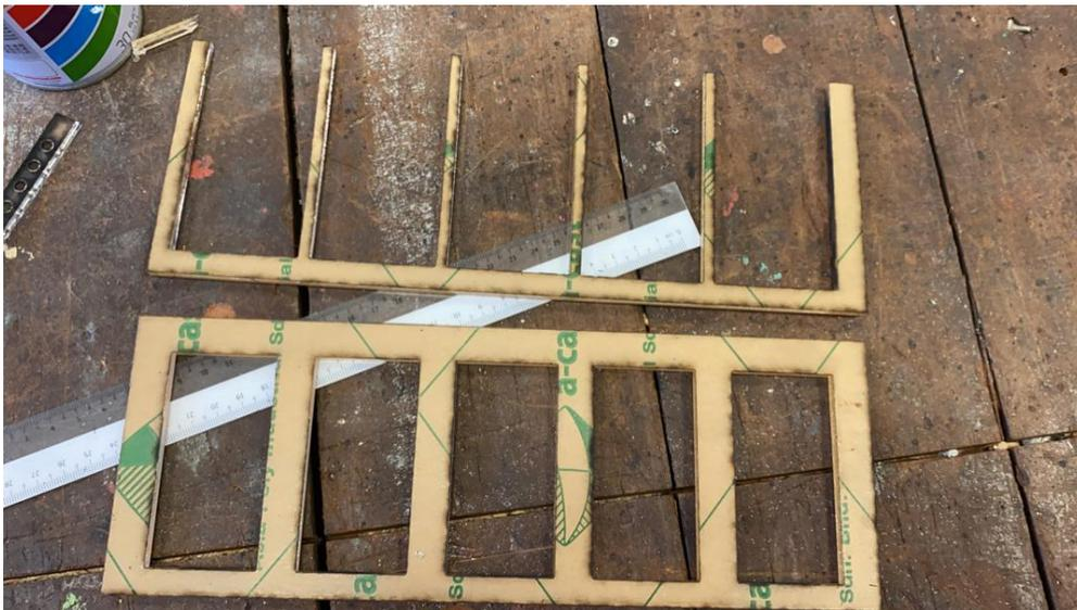
Figure 4-3 try fitting and dimension checking by ruler
