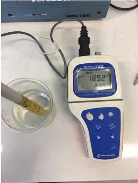
Figure 4-21 Electrical conductivity of  $\text{KOH } 1\text{mol/dm}^3$  before the discharge test, measured using electrical conductivity meter
