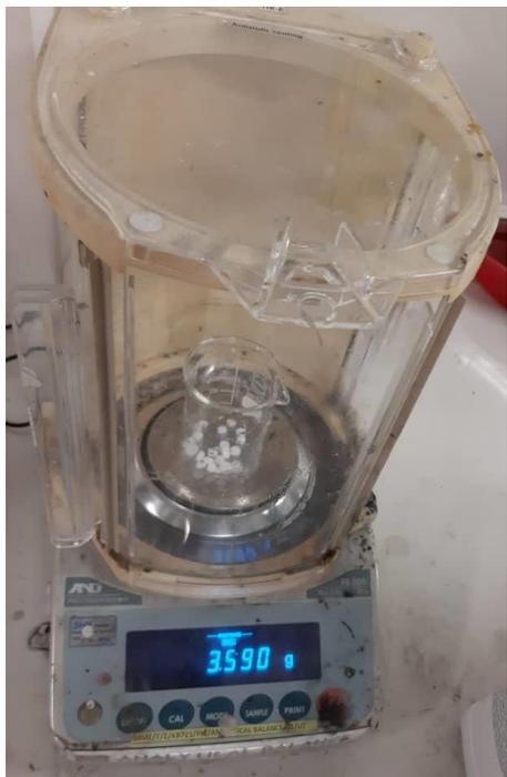
Figure 4-10 measuring NaOH in electrical scale with chamber to prevent air flow.
