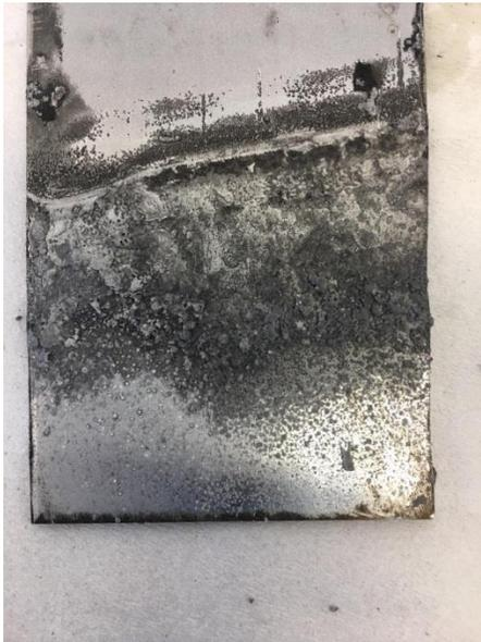
Figure 4-20 aluminium sheet after discharge test
