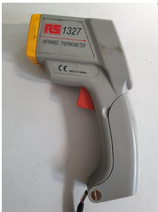
Figure 3.5 Infrared Thermometer for ensure Glow Plug is producing expected heat
