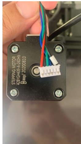
Figure 3.5: Stepper Motor Wiring
