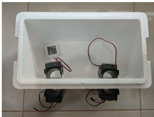
Figure 21: Inside view of chiller box
