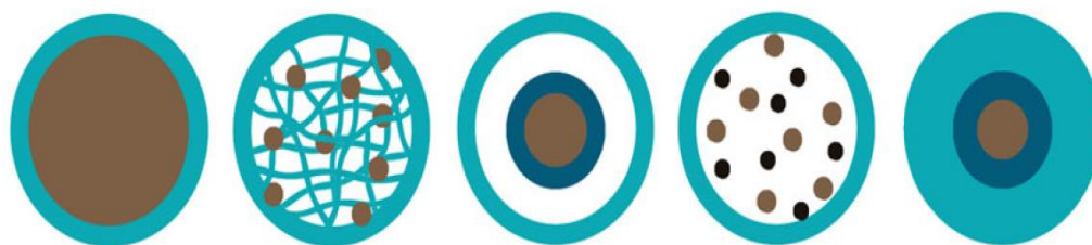
Figure 1.3: Schematic representations of the type of metallic-encapsulated polymer nanocomposites (from left to right): single-core capsule, dispersed core in a polymer gel, multi-layer capsule, dual-core capsule and single-core-multi-shell capsule (Sarabia and Maspoch, 2015)
