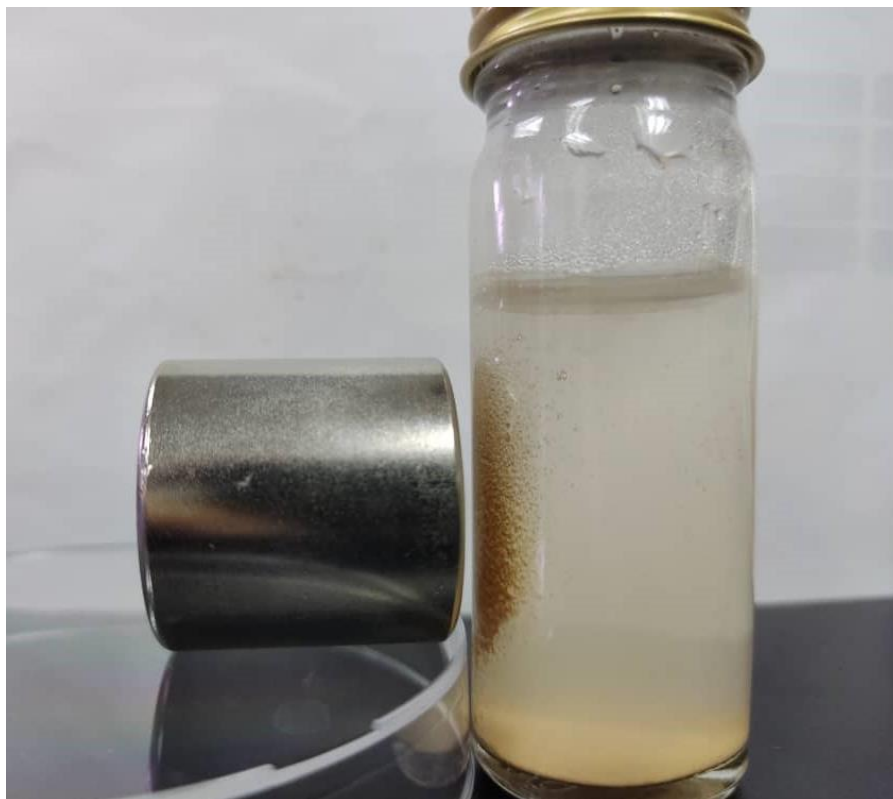
Figure 4.9: Magnetic recovery of \text{ZnO}/\text{BiOBr}/\text{MgFe}_2\text{O}_4 ternary composites after photocatalysis.
