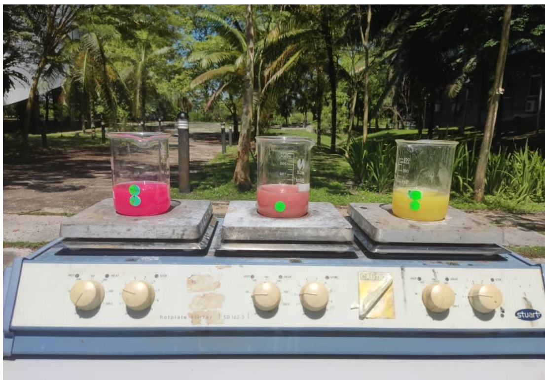
Figure 3.6: Experimental Setup for Photodegradation of Rhodamine B in aqueous solution
