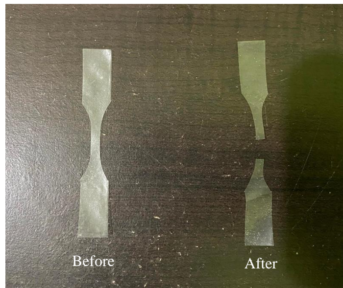
Figure A.31: Sample of the film before and after tensile test.
