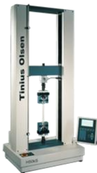
Figure 3.4: Tinius Olsen H10KS-0784 Tensile Testing Machine.
