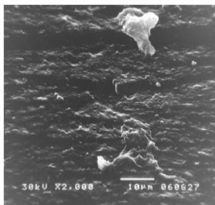
Figure 2.7: SEM Micrograph of NBR/EPDM rubber composite with 70 phr of carbon black (Jovanović, et al., 2013).
