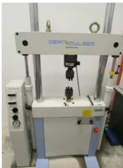
Figure 3.1: Shimadzu EHF-EM050K1-020-0A for Investigation of Tensile Properties of PVOH/CB composites.
