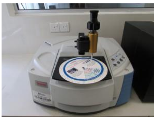
Figure 3.2: ThermoScientific Nicolet iS10 Fourier Transform Infrared Spectroscopy Used for Investigation of the Chemical Interaction and Bonding of PVOH/CB composites.
