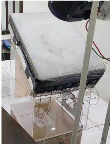
Figure A-7: Model of the Foam Concrete Roof with Moving Air Cavity and Solar Powered Fans (Roof Design V).
