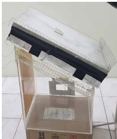
Figure A-6: Model of the Foam Concrete Roof with Moving Air Cavity (Roof Design IV).
