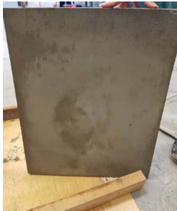
Figure A-1: Lightweight Foam Concrete Ready for Curing Process.
