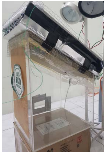
Figure A-8: Model of the Foam Concrete Roof with Moving Air Cavity, Solar Powered Fans and Rockwool (Roof Design VI).
