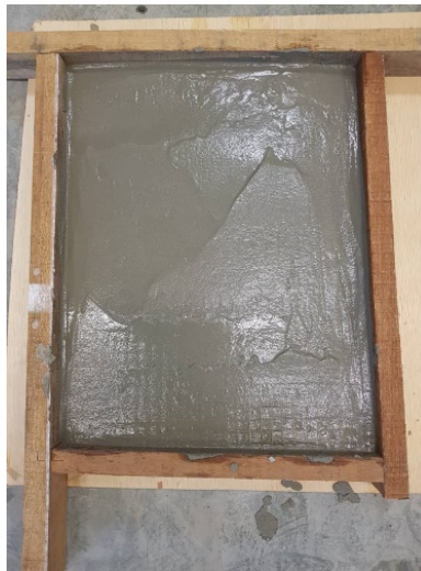
Figure 3.3: The Lightweight Foam Concrete Tile in a Mould.
