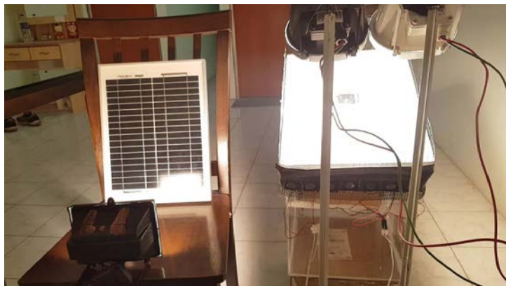
Figure 3.11: The Solar Panel and Solar Powered Fans Set Up.
