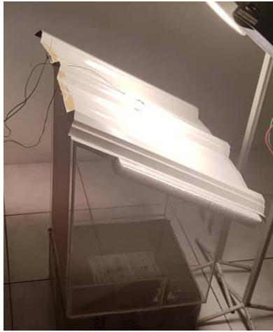
Figure A-4: Model of the Metal Deck Roof with Thermal Reflective Coating (Roof Design II).
