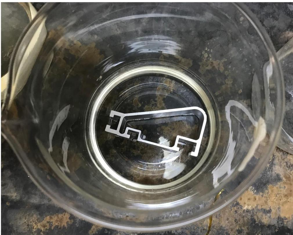
Figure 3.5: Aluminium Extruded Product (4824) Immersed into Desmutting Solution (40% Nitric Acid and 60% Distilled Water).
