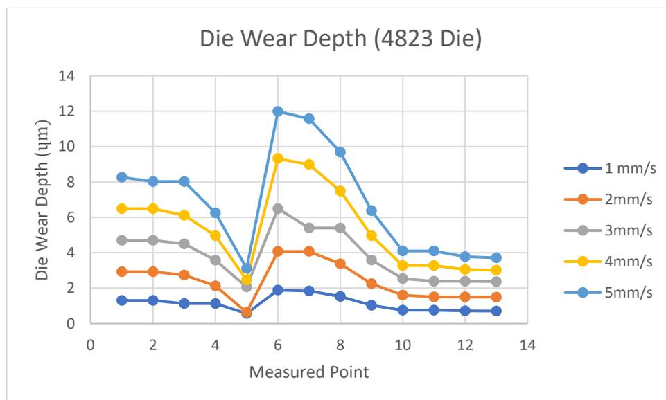
Figure 4.29: Distribution of Die Wear Depth on Measured Points at Different Ram Speed (4823 Die).
