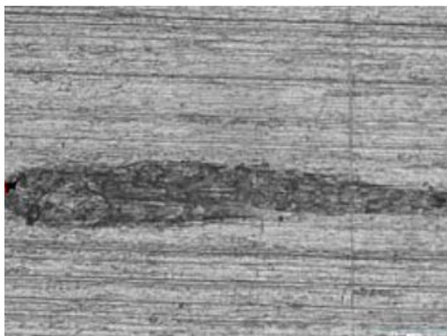
Figure 2.20: Pick-up Defect (Fourmann, 2017).
