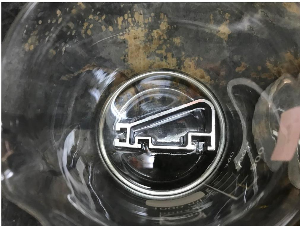
Figure 3.3: Aluminium Extruded Product (4824) Immersed in Acetone Solution.
