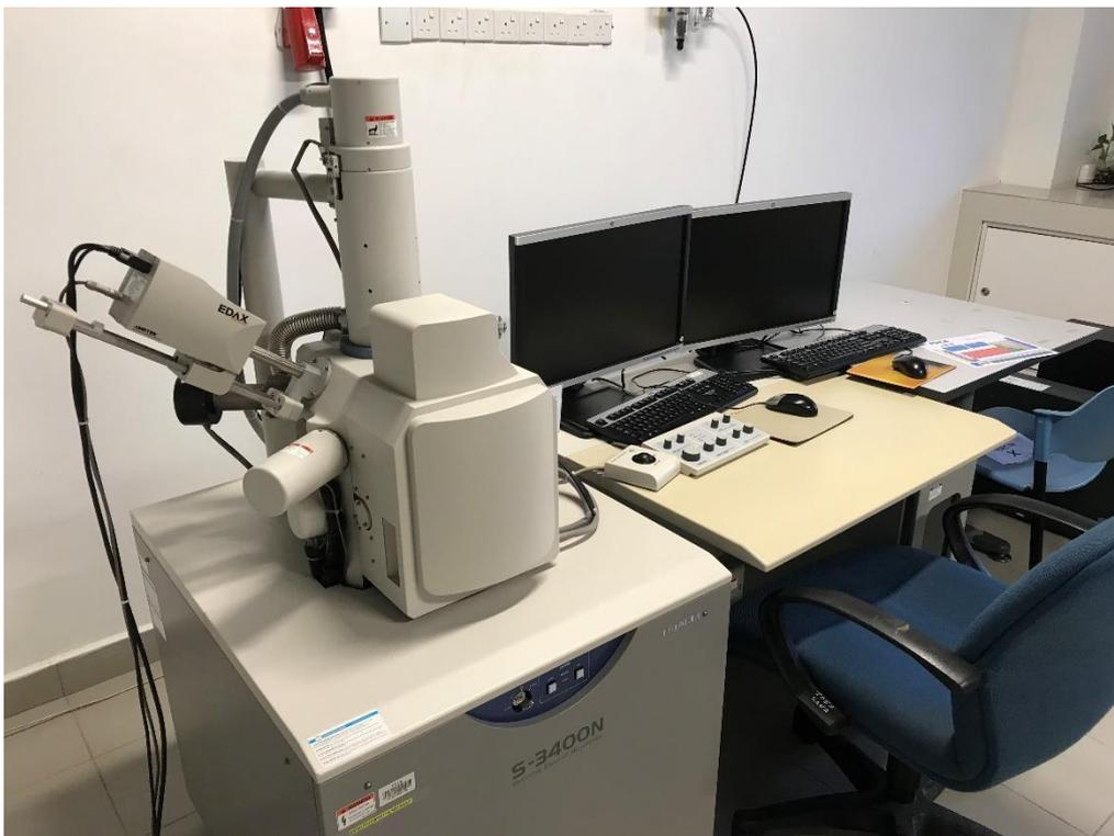
Figure 3.9: Scanning Electron Microscope (SEM) with Energy Dispersive X-ray (EDX) Analysis.
