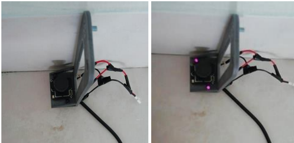
Figure A 2 Illumination of IR LED on Camera Arm
