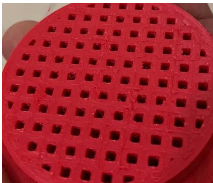
Figure 4.3.4 : Printed Cartesian panel.
