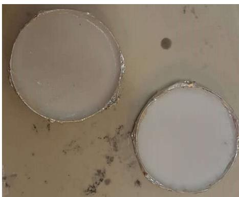
Figure 3.4: Liquid form of  $H_3PO_4$  gel electrolyte after 5 hours of mixing.
