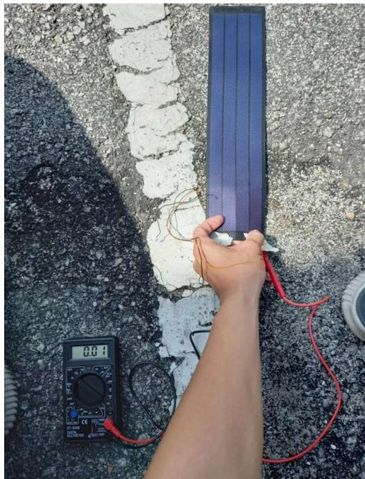
Figure 3.8: Photo shows the method used to charge EDLCs with solar PV, where the multimeter is parallel to the circuit of solar PV and EDLC to measure the voltage provided by the solar PV to EDLC.
