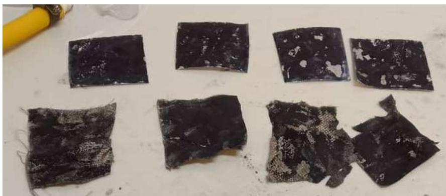
Figure 3.3: Photo of activated carbon coating applied on silver coated clothing (2nd row) and aluminium sheet (1st row) for the 1st time.
