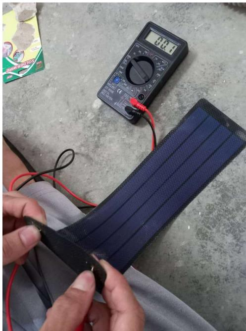
Figure 3.6: Measurement on flexible solar PV using multimeter.
