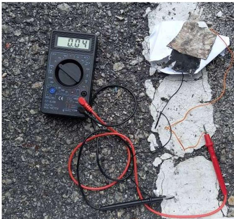
Figure 3.9: Photo shows the method used to measure the discharge EDLCs using multimeter.
