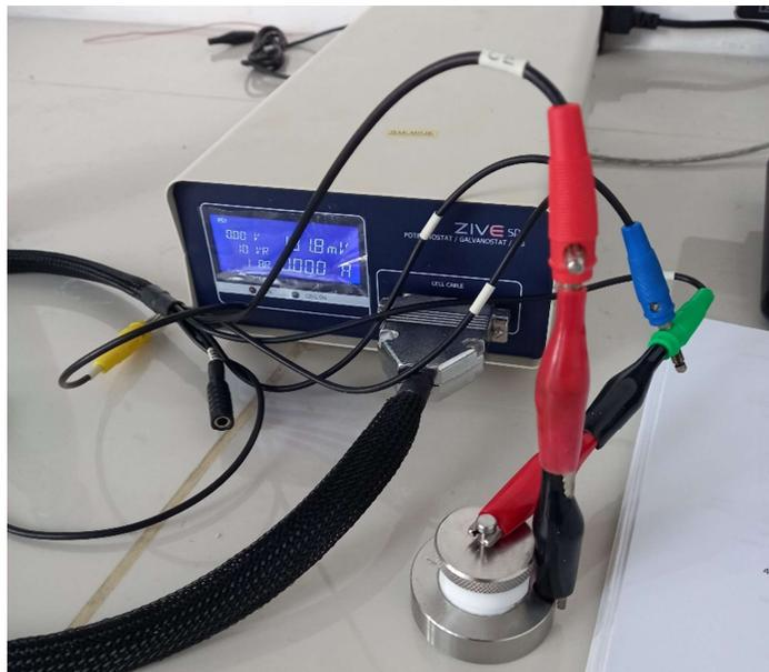
Figure 3.7: Figure shows EIS conducted on PVA gel electrolyte measured with ZIVELAB potentiostat.
