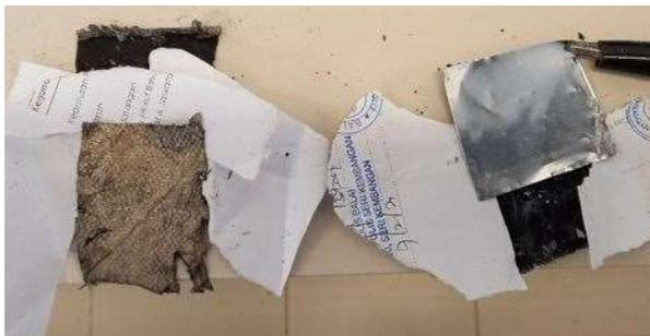
Figure 3.5: Figure illustrates fabricated EDLCs made of silver cloth (left) and aluminium sheet (right).
