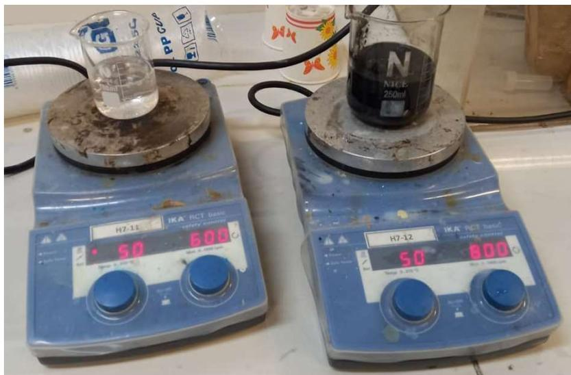
Figure 3.2: Picture illustrates mixing of activated carbon coating (right) and PVA gel (left).
