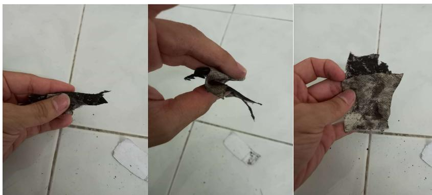
Figure 4.5: Silver coated textile EDLC is rolled into round shape (Left 1) and bent 90 degrees (Left 2), the shapes of the EDLC still retains without any damage (Left 3).
