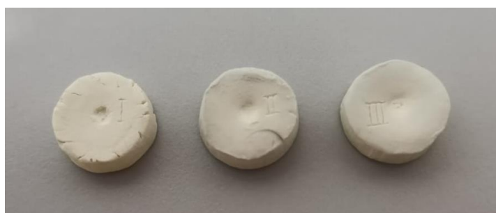
Figure 4.15: Three samples after sintered, binders used for sample I: CMC, II: HPMC, III: MC
