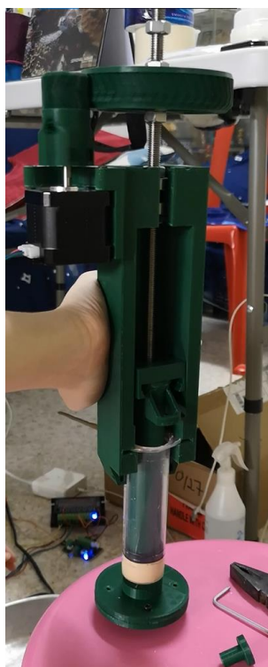
Figure 3.19: 3D-Printed Syringe Pump Extruder
