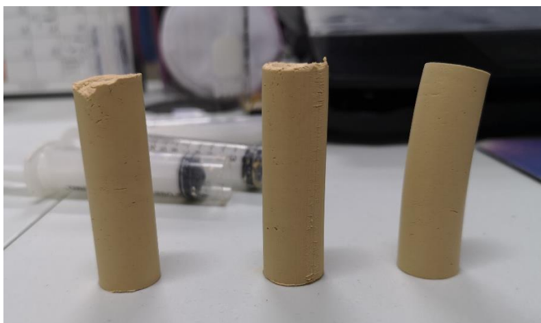
Figure 4.6: Clays using MC (hard, medium and soft arrangement from left to right)
