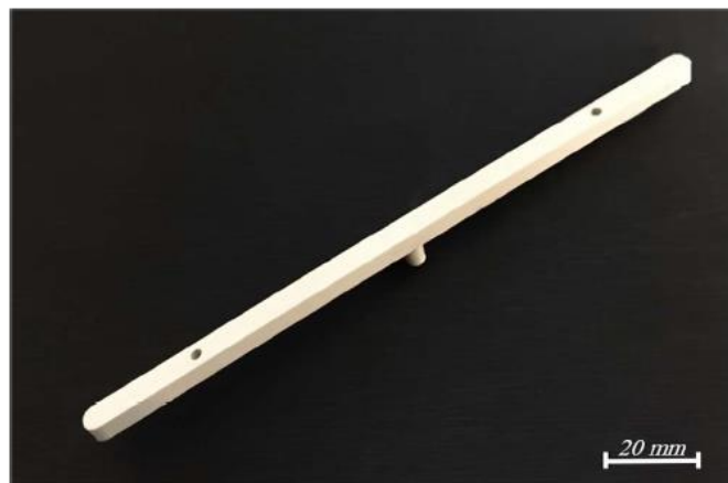
Figure 2.5: Injection Moulded Part (Green Part) (Sardarian, Mirzaee and Habibolahzadeh, 2017a)
