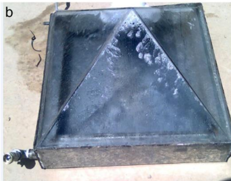
Figure 2.11 : Solar distiller with pyramid-shaped glass cover (Taamneh and Taamneh, 2012).
