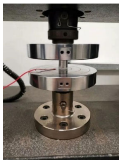
Figure 3.5: Experimental Setup of Compressive Test (Tam, 2019)
