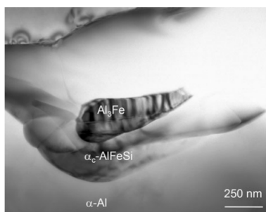
Figure 2.14: TEM image revealed an Al 3 Fe particle embedded within \alpha_c -AlFeSi phase in the AA6060 alloy with Fe of 0.5 wt%(Sweet et al., 2011).
