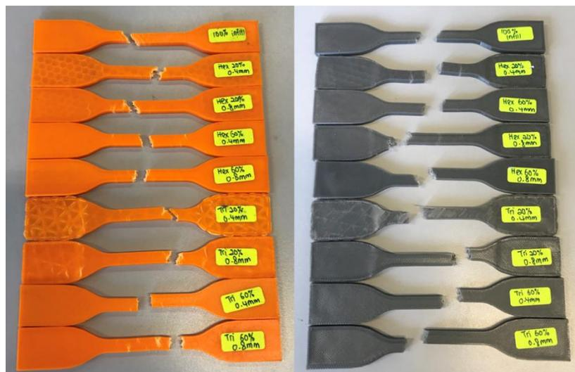
Figure 3.8: Tensile tested specimens of PLA and PETG
