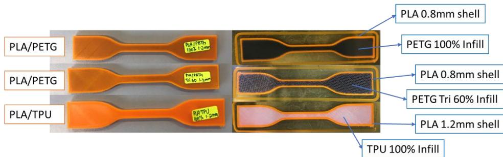
Figure 3.6: Composites tensile test sample fabricated
