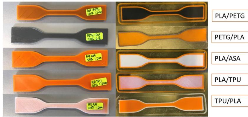
Figure B-1: The composites sample fabricated
