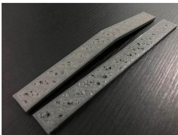
Figure 4.12: Bad surface finish on the top shell
