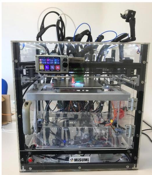
Figure B- 3: Multitools 3D printer used for sample fabrication
