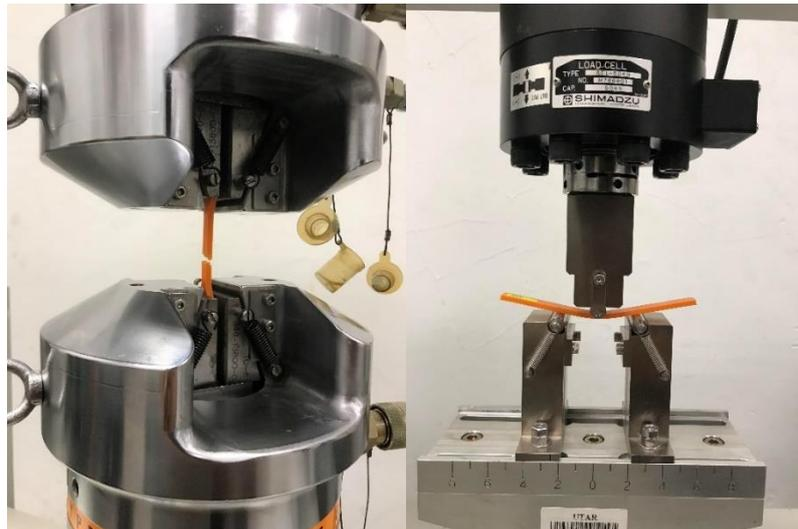
Figure 3.7: Test setup for determining the tensile properties (left) and flexural properties (right)
