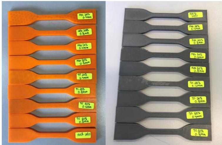
Figure 3.4: Tensile test samples 3D printed with PLA (orange) and PETG (grey)
