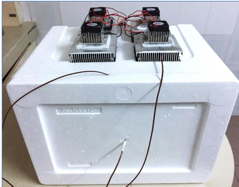
Figure 3.5: Chamber design for heating mode
