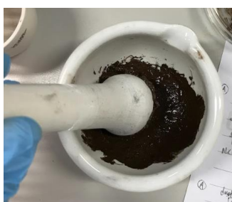
Figure 3.7: The Treated EAFD and \text{NiCl}_2 \cdot 6\text{H}_2\text{O} were Mixed and Ground in the Mortar.
