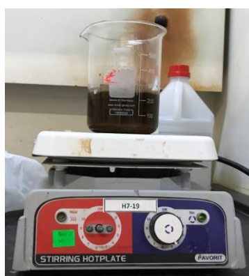
Figure 3.4: The Mixture of the EAFD with the Diluted HCl (0.5 mol/L ) Solution in the Beaker Placed on the Electromagnetic Stirrer.
