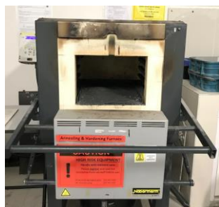
Figure 3.8: Annealing and Hardening Furnace (Nabertherm K4/13) Used in this Project.
