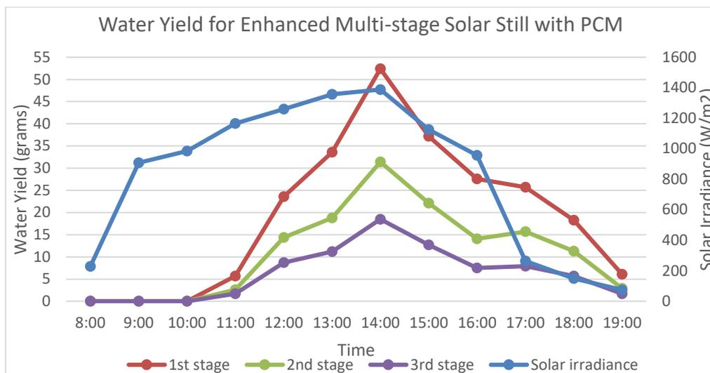
Figure 4.12: Graph of water yield for enhanced multi-stage solar still with PCM
