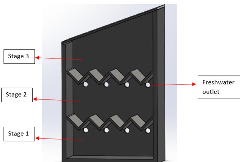
Figure 3.15: Section view of the v-corrugated multi-stage solar still
