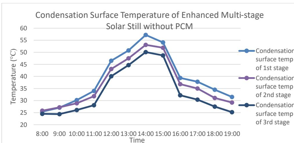
Figure 4.6: Graph of condensation surface temperature of enhanced multi-stage solar still without PCM
