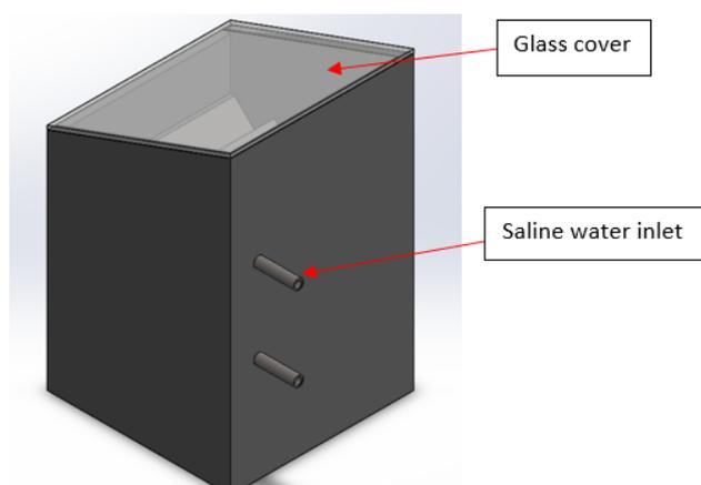
Figure 3.16: Isometric view of v-corrugated multi-stage solar still
