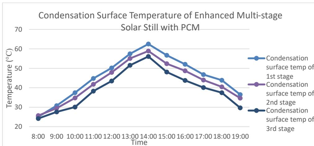
Figure 4.8: Graph of condensation surface temperature of enhanced multi-stage solar still with PCM
