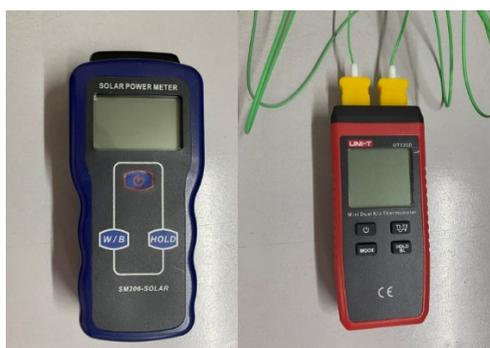
Figure 3.19: Solar meter (left) and type K thermocouple (right)
