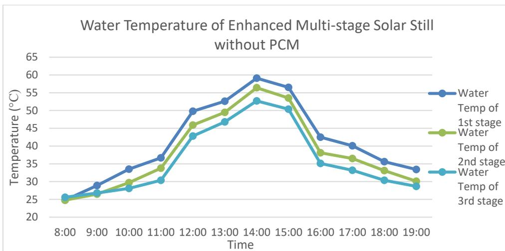
Figure 4.5: Graph of water temperature of enhanced multi-stage solar still without PCM
