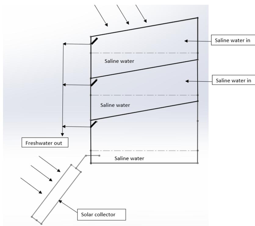
Figure 3.7: Inclined flat condensation surface
