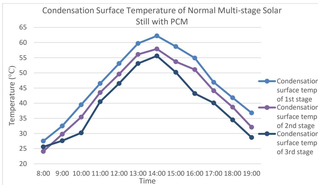
Figure 4.4: Graph of condensation surface temperature of normal multi-stage solar still with PCM
