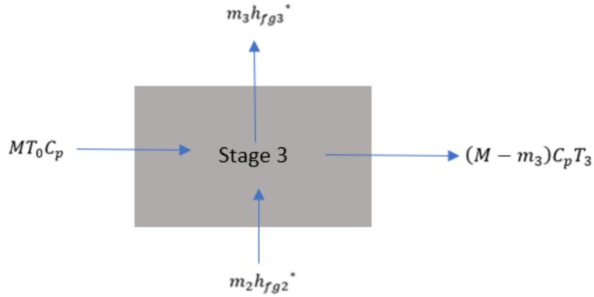
Figure 3.2: Heat balance in stage 3
