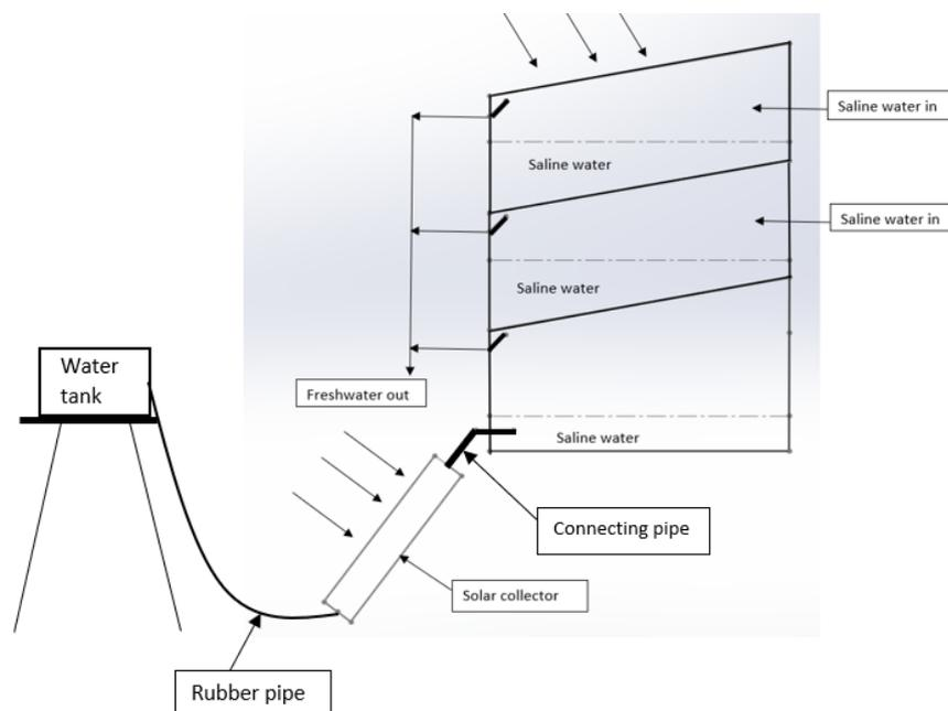
Figure 3.13: The detailed experiment setup
