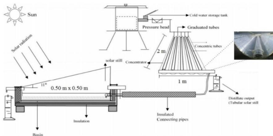
Figure 2.2: Parabolic concentrator in single slope solar still
