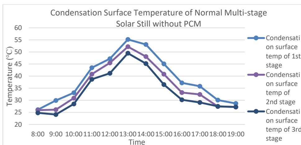
Figure 4.2: Graph of condensation surface temperature of normal multi-stage solar still without PCM
