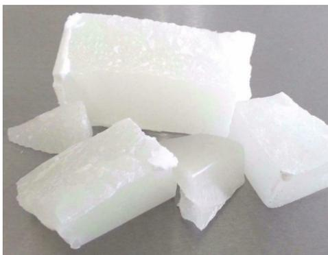
Figure 3.6: Paraffin wax as PCM used in multi-stage solar still
