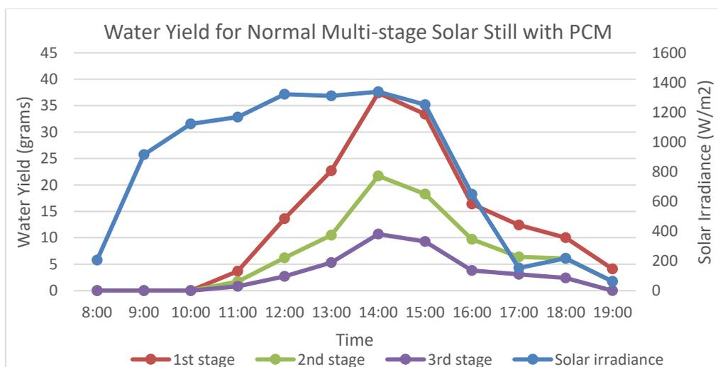
Figure 4.10: Graph of water yield for normal multi-stage solar still with PCM
