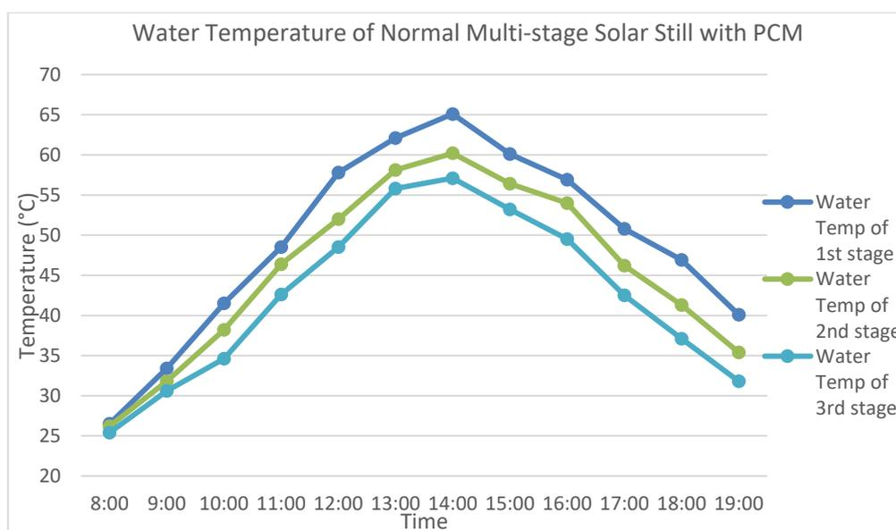
Figure 4.3: Graph of water temperature of normal multi-stage solar still with PCM
