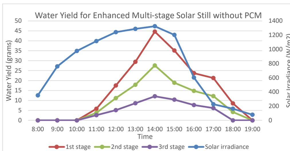
Figure 4.11: Graph of water yield for enhanced multi-stage solar still without PCM
