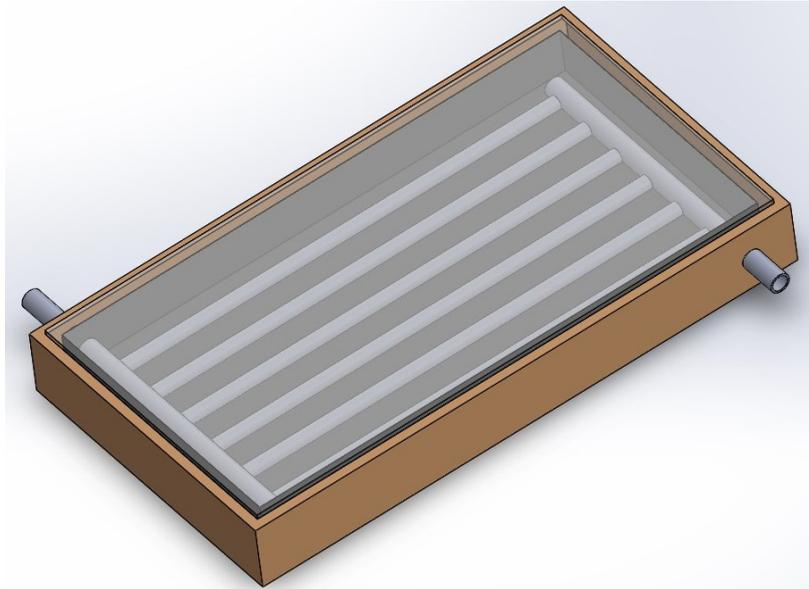
Figure 3.12: Design of flat plate solar collector
