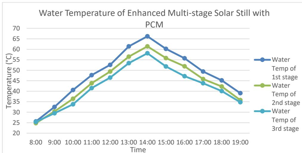
Figure 4.7: Graph of water temperature of enhanced multi-stage solar still with PCM
