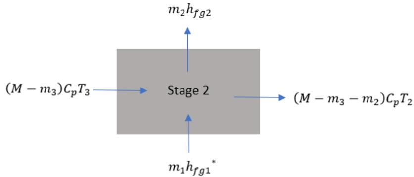
Figure 3.3: Heat balance in stage 2
