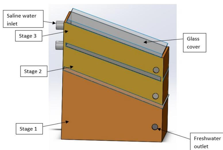
Figure 3.14: The inclined surface of three-stage solar still design
