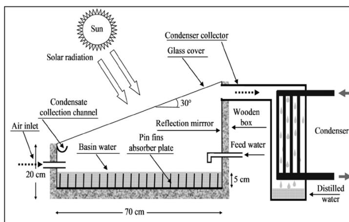
Figure 2.8: Pin fin still with condenser (Rabhi et al., 2017)
