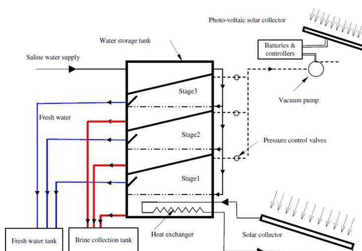
Figure 2.5: Three-stage evacuated solar still with heat exchanger (Ahmed et al., 2009)
