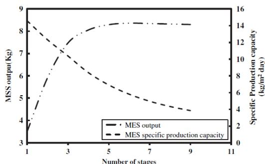
Figure 2.4: Result of output (kg) and the number of stages (Younas et al., 2016)
