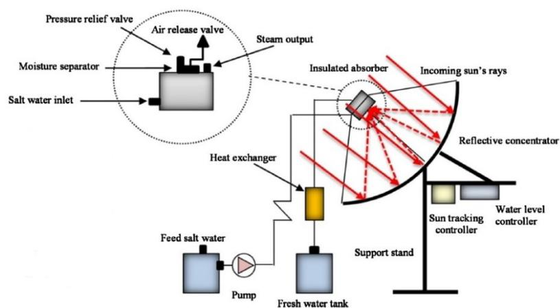
Figure 2.1: Parabolic concentrator solar distiller design (Gorjian et al.,2014)
