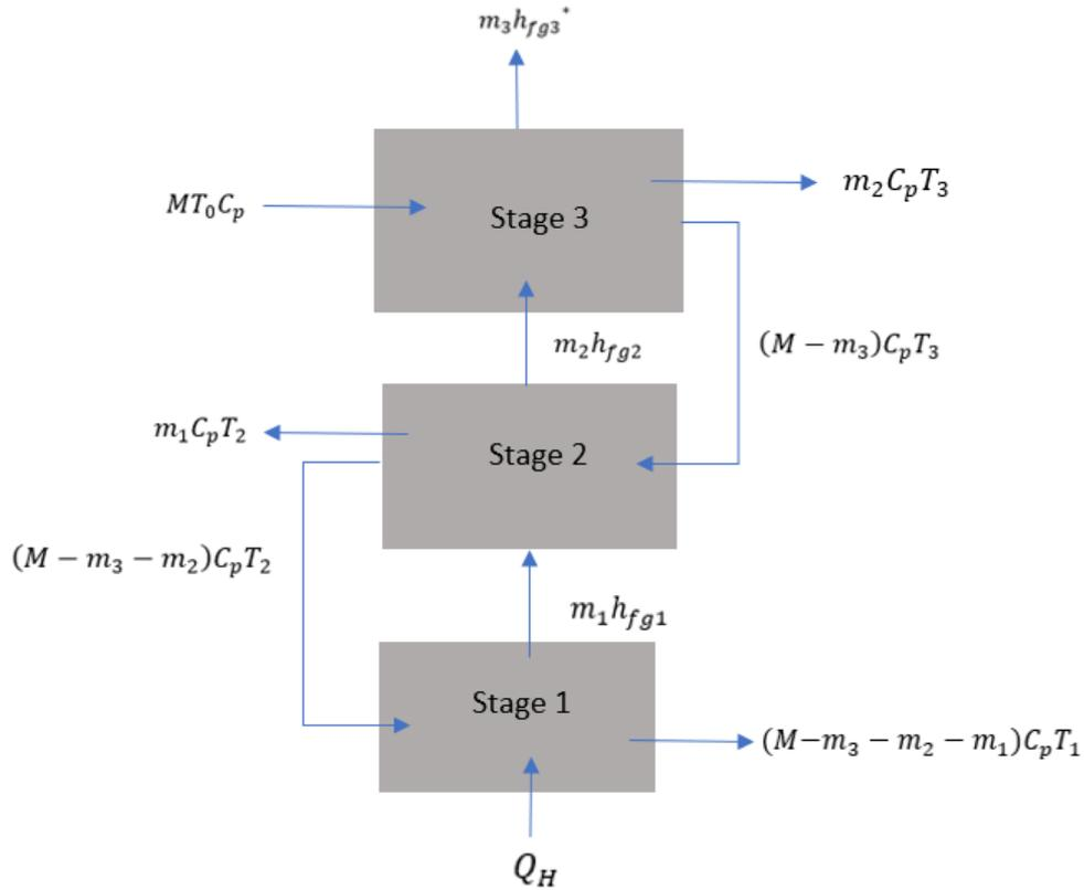
Figure 3.5: Total energy flow through the solar still
