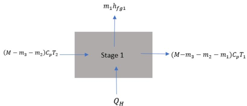
Figure 3.4: Heat balance at stage 1
