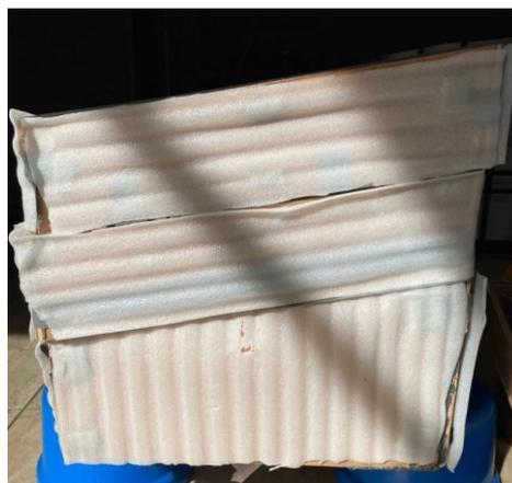
Figure 3.17: Multi-stage solar still with flat plate condensation surface
