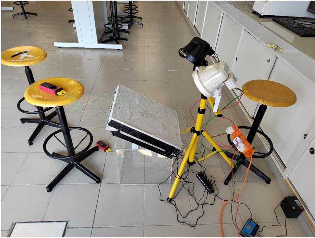
Figure A-5: Roof Model IV (LFC Roof Slab with Active MAC Fitted with S-P Fs).
