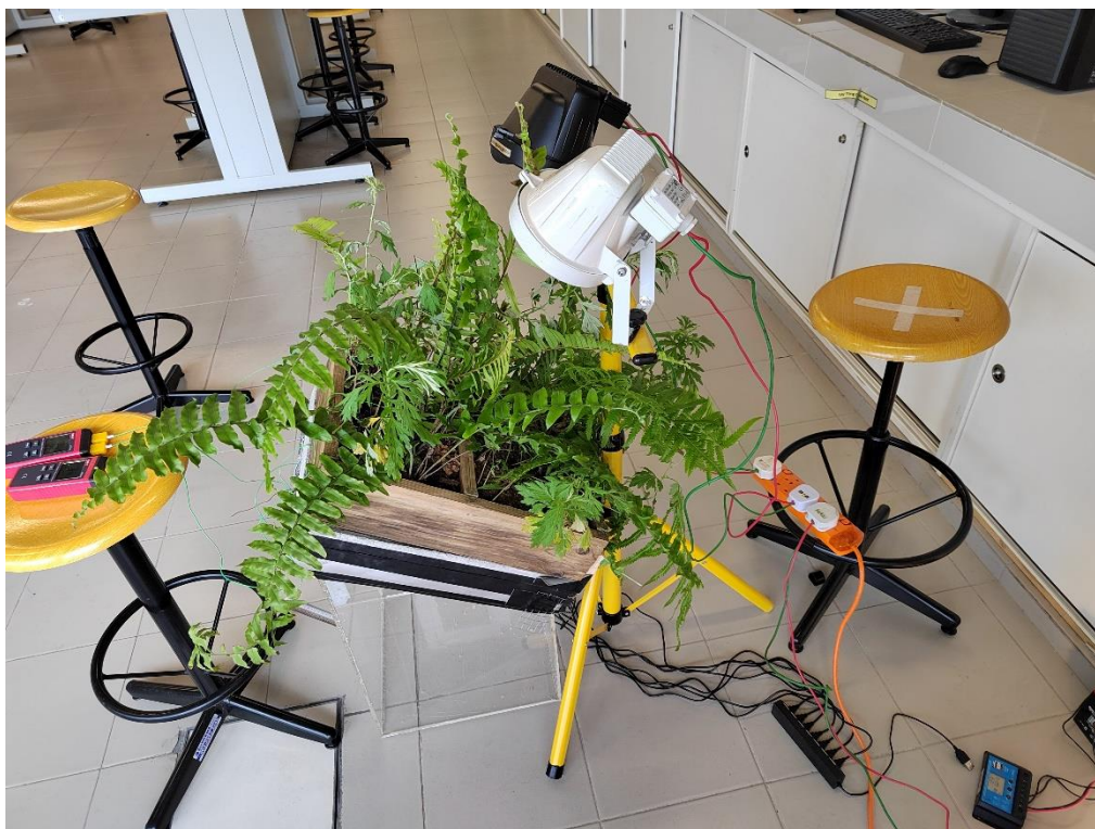
Figure A-7: Roof Model V (LFC Roof Slab Topped with Vegetation Layer with Active MAC Fitted with S-P Fs).
