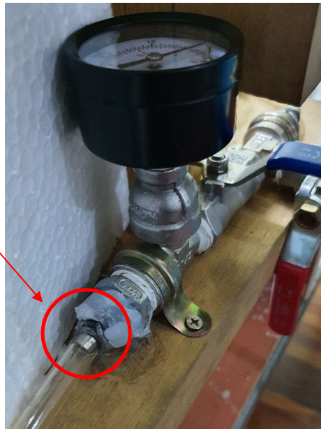
Figure 3.11: Exit of fitting towards evaporator.
