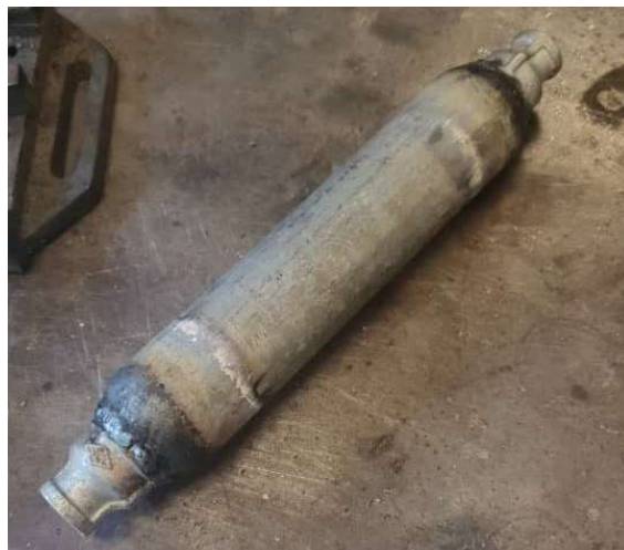
Figure 3.5: GI pipe with welded GI sockets.
