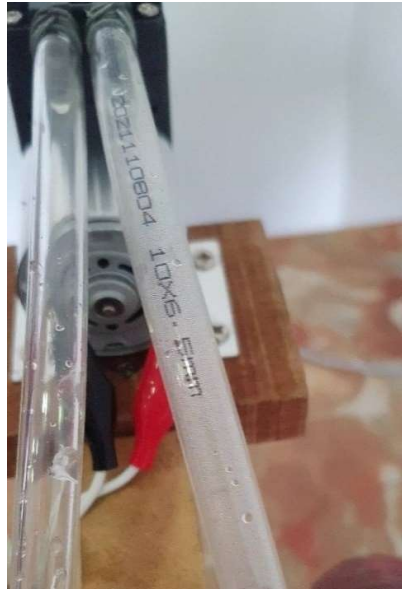
Figure 4.5: Condensate forming in transport line heading towards condenser.
