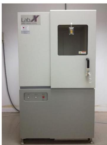
Figure 3.3: X-ray Diffractometer.
