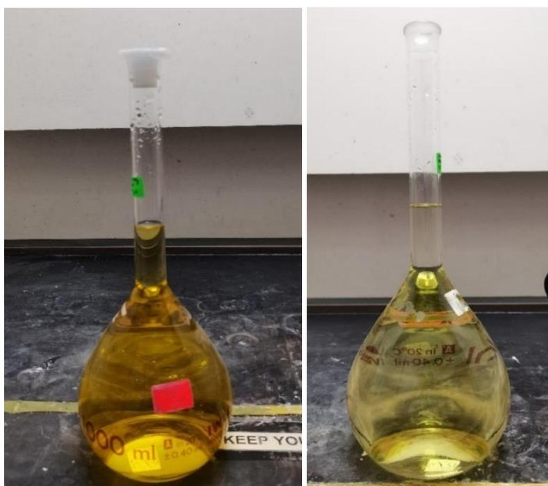
Figure 3.4: 100 mg/L (left) and 10 mg/L (right) of Cr (VI) Solution Prepared in Volumetric Flasks.
