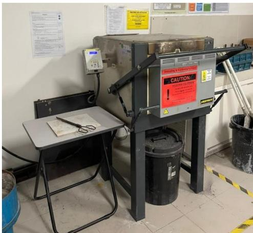
Figure 3.1: Muffle Furnace.
