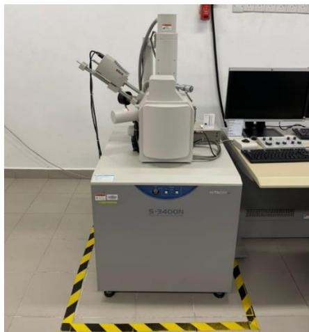
Figure 3.2: Scanning Electron Microscope (Hitachi S-3400N).
