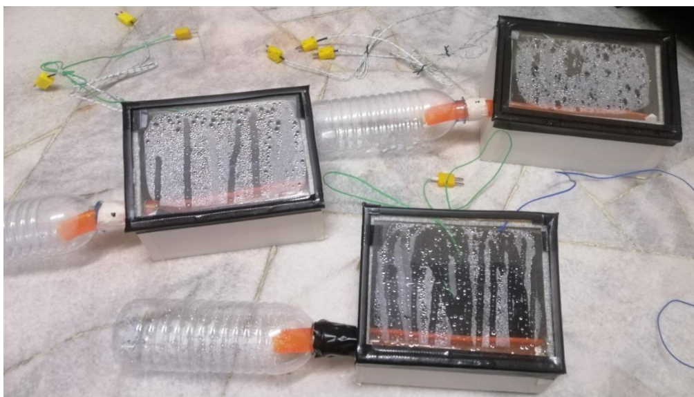
(upper left corner: model with paraffin wax, middle: model without PCM, upper right corner: model with soft paraffin)
