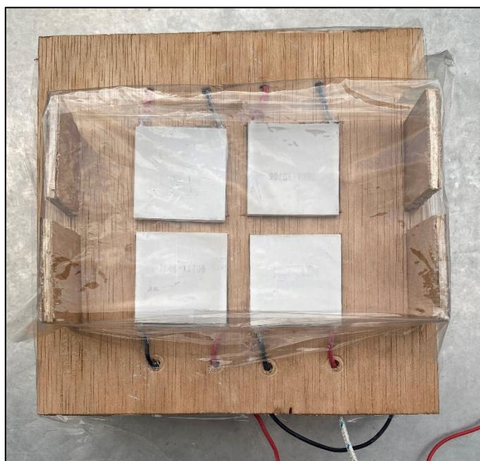
Figure 3.14: Prototype with \text{TiO}_2 coating
