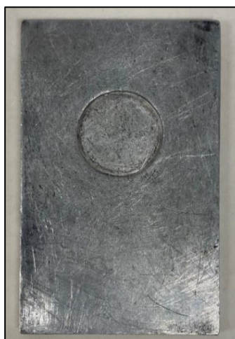
Figure 3.6: Mould for \text{SiO}_2 and \text{TiO}_2 powder
