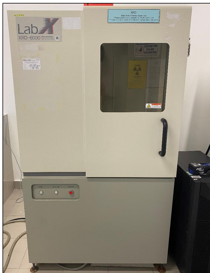
Figure 3.5: Shimadzu XRD-6000 X-ray Diffractometer
