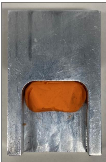
Figure 3.7: Mould for \text{SiO}_2 and \text{TiO}_2 samples
