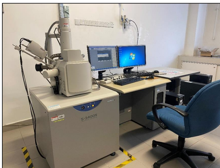
Figure 3.9: Hitachi S3400-N SEM-EDX Machine
