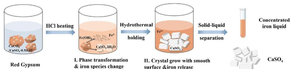
Figure 2.25: Overall Mechanism of Removing Iron from Red Gypsum (Peng, et al., 2021).
